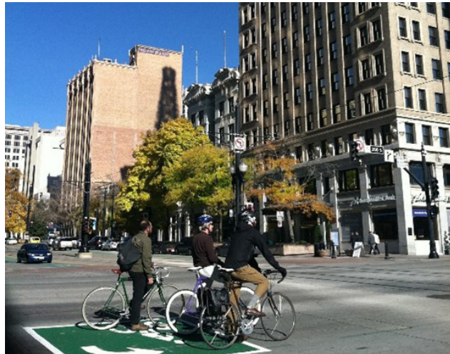
Two-Stage Turn Queue Box A designated area for cyclists to queue while waiting to turn.
