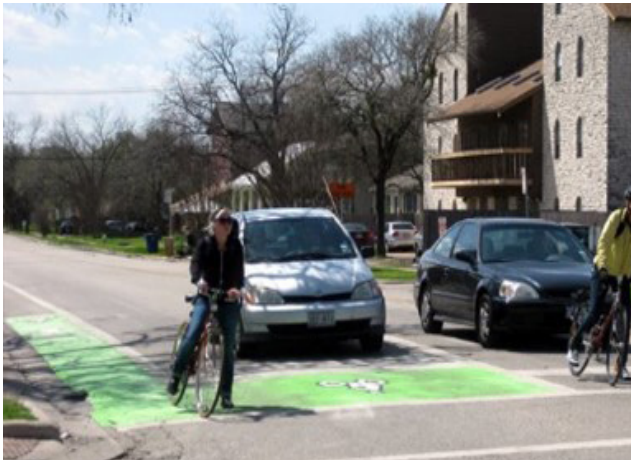
Bike Box A designated area at the head of a traffic lane at a signalized intersection that provides bicyclists with a safe and visible way to get ahead of queuing traffic during the red signal phase.
